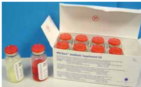
Reagent 1: Lyophilized antibiotic cake Reagent 2: Reconstitution fluid NOTE: Rehydrate powder with 10 ml reconstitution fluid and discard unused portion 7 days after rehydration.
