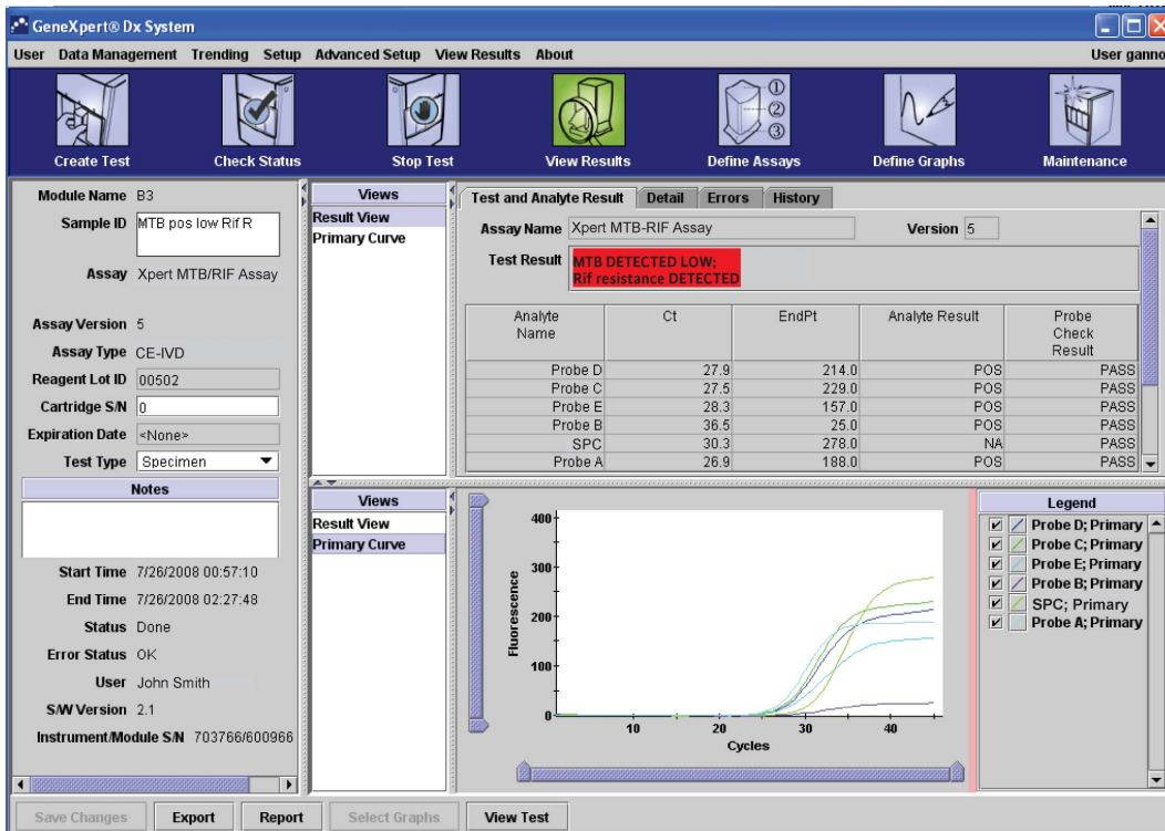
Figure 2. GeneXpert Dx System—Privileged User View Results window, MTB Detected Low, Rif Resistance DETECTED
