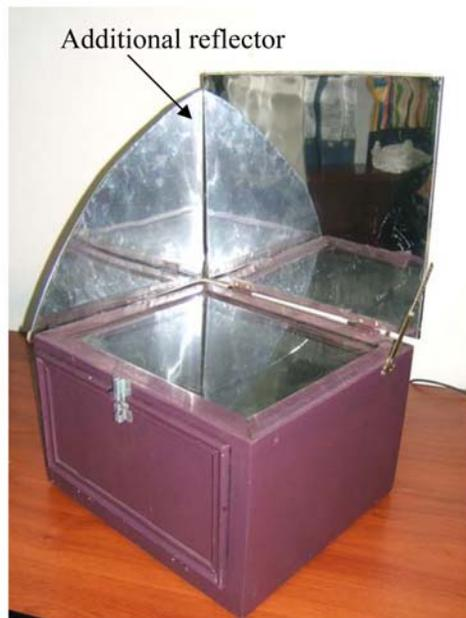
**Figure 1.** Box type solar cooker used in this study (A) original design (left) with control box (right) and (B) final design with additional reflector.
