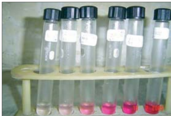
Figure 3: A reference standard for visual reading of the color intensity was prepared by serial two fold dilution of 1:128 dilution of Sodium nitrite ( \text{NaNO}_2 ) stock solution (10 mM \text{NaNO}_2 ). The standard tubes are graded from 1+ through 6+ (From left to right)
